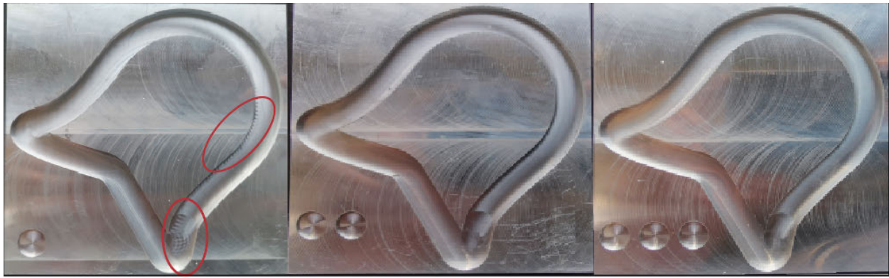
Fig. 10. Milling results from left to right: risk bound, safe bound, fuzzy bound.
